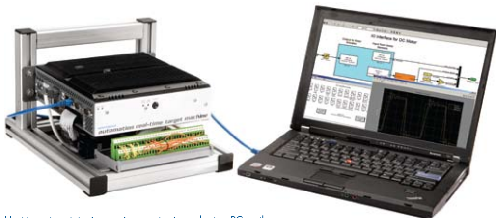
Host-target prototyping environment using a laptop PC as the host computer and an industrial PC as the real-time target.
