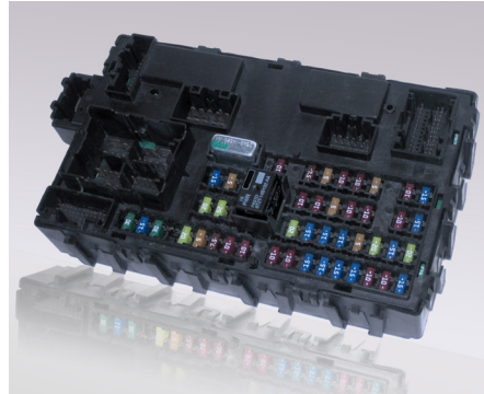
Lear automotive body electronic control unit.
