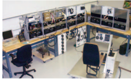
Hardware-in-the-loop truck simulator.
