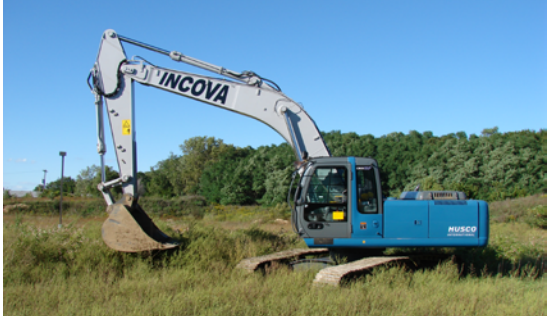
A 25-ton excavator with hydraulic functions controlled by HUSCO’s INCOVA system.
